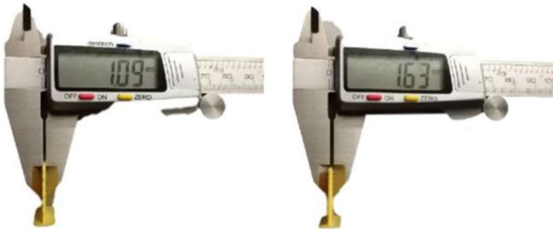
Fig. 2 Error due to filament diameter variations
