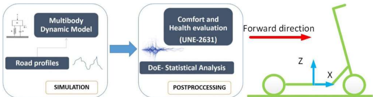
Fig. 1 Methodology scheme and e-scooter layout
