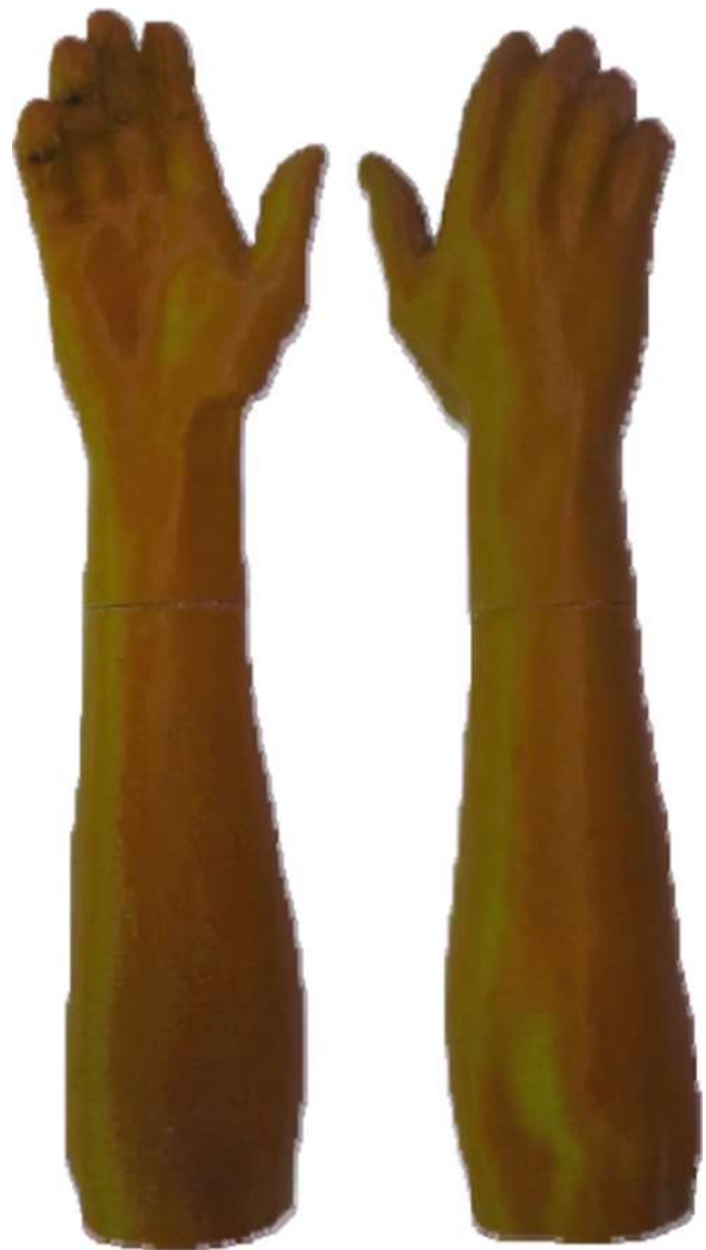
Fig. 24 PLA printed arm
